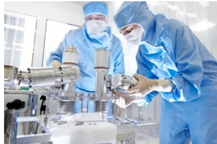
Power coupler preparation in clean room
