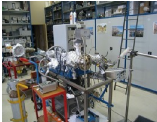
Setup for degazing rate measurement
