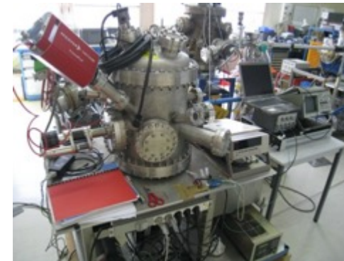
Setup for desorption and SEY measurement
